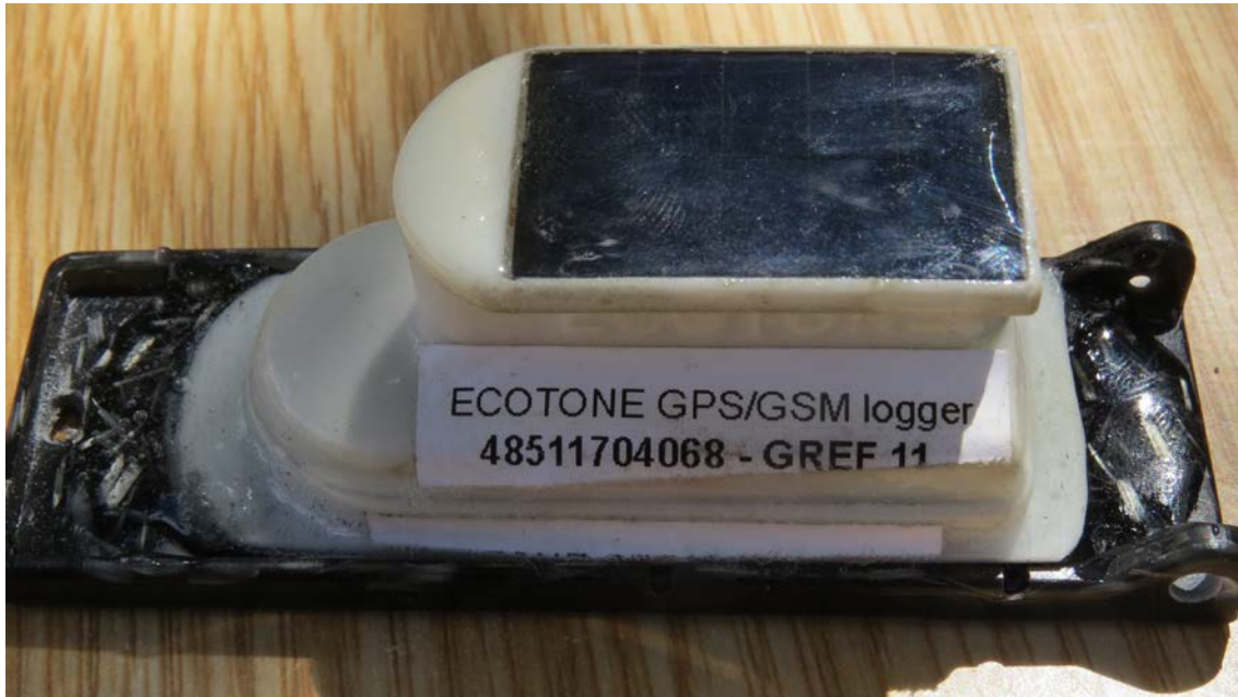
Photo 19. Detail of a GPS-GSM transmitter used in 2014. Photo: Gerard Plana.
